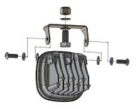
14. With the 9/16" wrench and socket, mount the lights onto the brackets as shown in the driver's side picture below. Repeat steps for the passenger side. Remove harness attached to the front facia and set aside. It will not be reused.
