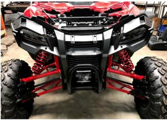
8. The bottom portion of the front fascia must now be moved to free the entire front end. Take care not to damage the bottom mounts of the fascia, or the radiator side cover shown in step six. Remove the Fascia and place it face down on a soft non-marking surface.
