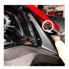
4. Remove the plastic fastener on the left below. With a 5mm allen wrench, remove the circled fastener below. Repeat for passenger side.
