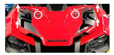
2. With a 10mm Socket Wrench, remove the four bolts arrowed below.
